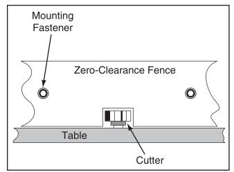
Figure 20. Example of a zero-clearance fence.
